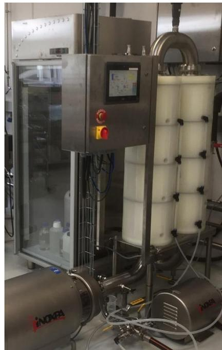
A 20 m<sup>2</sup> Hollow Plate™ cross flow plant
