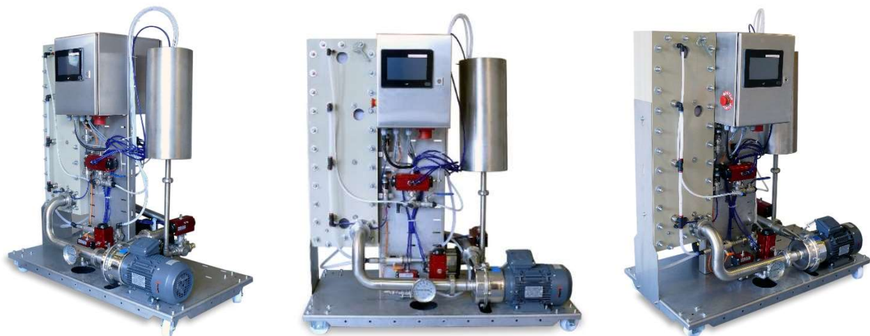
The PLC controlled Pilot Plant
